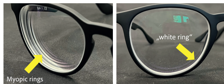
Fig. 2: Myopic rings and “white rings” affect the overall appearance of the spectacles. Example glasses with -4dpt lenses.
